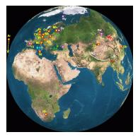
And... the EVN + VLBA can even operate with space-based radio telescopes, giving an effective aperture of 20,000km! This gives resolutions of just micro-arcseconds. (something 1mm across on the surface of the moon would have an angular size of 1 micro-arcsecond!)
