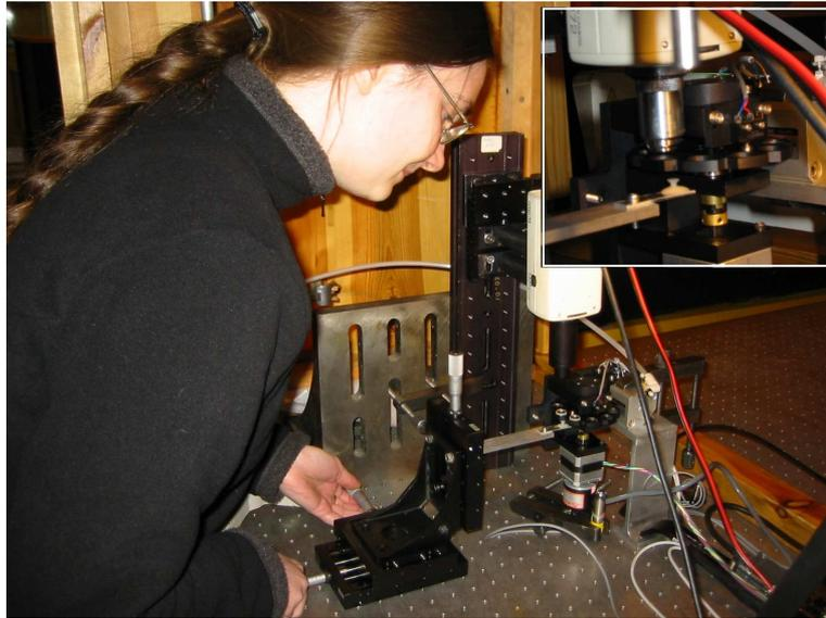
Figure 4.32: Optical bench in the Aluminising area of the WHT set-up for the focal mask alignment and gluing procedure. The up-ended table clamped to the bench was an improvisation for a projection screen as the ceiling is extremely high in this area. A picture of the complete set-up is shown in Figure A.2.
