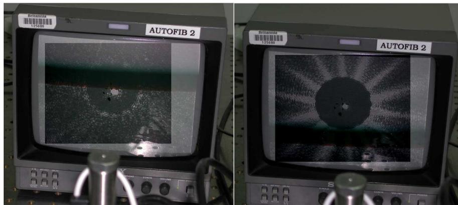
Figure 4.17: TV monitors relaying an image of the OSCA focus at the test-bench of the WHT. On the left is the focus with the 2 arcsec occulting mask in place and the Lyot stop. The picture on the right is the same set-up but with the Lyot stop removed. The effectiveness of the Lyot stop in removing the bright diffraction pattern is clearly demonstrated.
