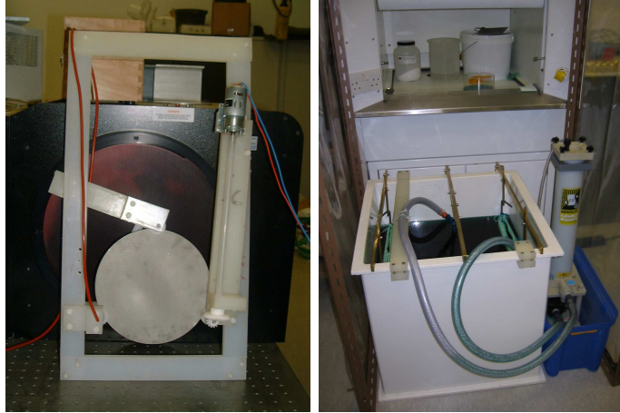
Figure 3. (Left) The spinning electrode mechanism. The titanium electrode contact is on the bottom left of the rig, with the motorised roller on the bottom right to spin the mirror. (Right) The nickel sulphamate electroplating tank into which the entire mirror rig is immersed and connected to the brass cathode.
