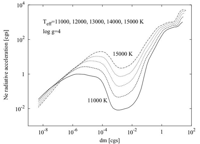
**Figure 4.** Radiative accelerations on Ne throughout the atmosphere as a function of stellar effective temperature and depth. Calculated for standard abundance of Ne.
