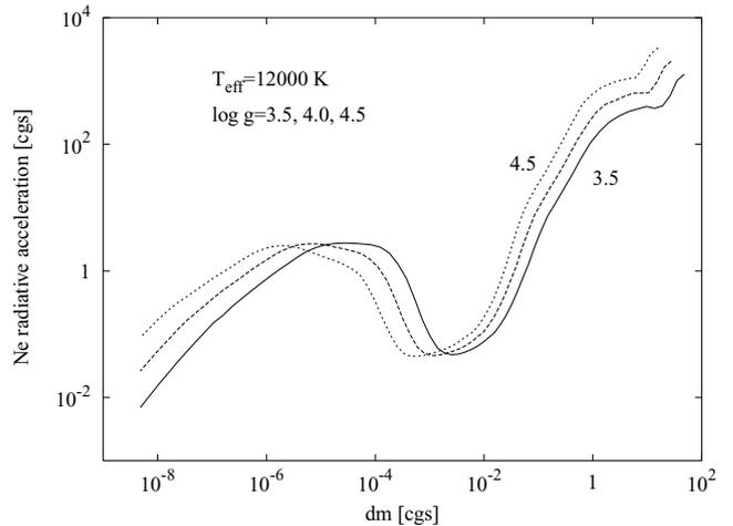
**Figure 5.** Radiative accelerations on Ne throughout the atmosphere as a function of stellar surface gravity and depth. Calculated for standard abundance of Ne.
