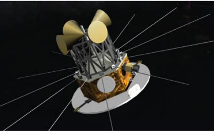
2<sup>nd</sup>-gen. prototype to be deployed Oct. 2013 in Green Bank – larger biconical antenna with higher gain at low frequency, improved
