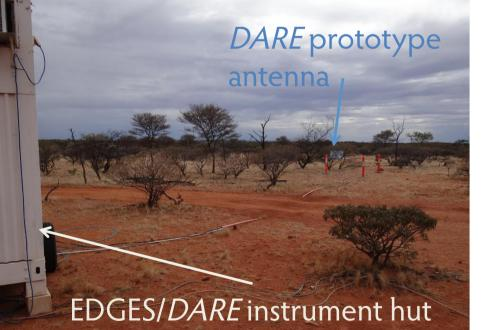
Prototype was deployed at MRO site in Western Australia; fewer problems with FM, but low-frequency RFI (probably naval radar) required extra filters and attenuation.
