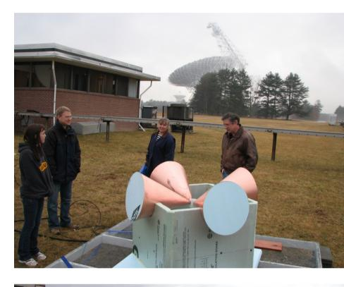
1<sup>st</sup>-gen prototype testing in Green Bank; Mar. 2012. Validated antenna, front-end and spectrometer performance and showed effects of ionosphere and RFI (especially FM band).
