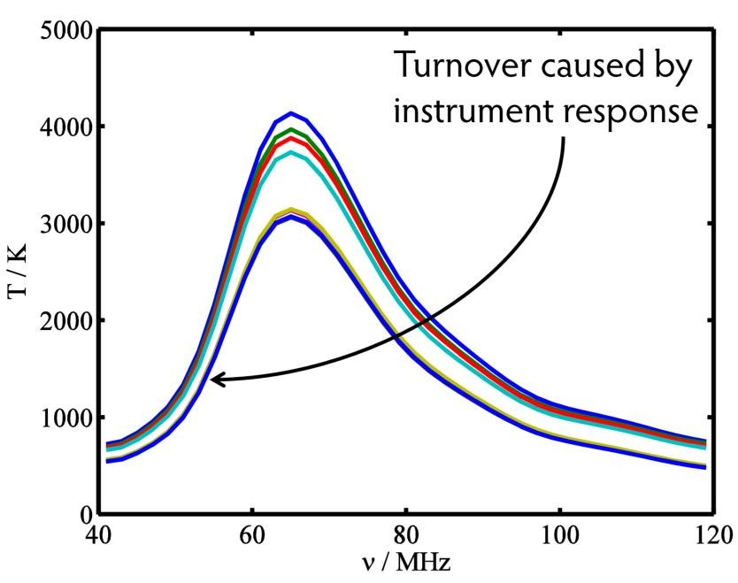
Noisy synthetic spectra from 8 DARE pointings (total 3000 h, or ~3 yr mission). DARE's large beam allows us to measure ~8 independent spectra (different foregrounds but same signal) from different directions.
