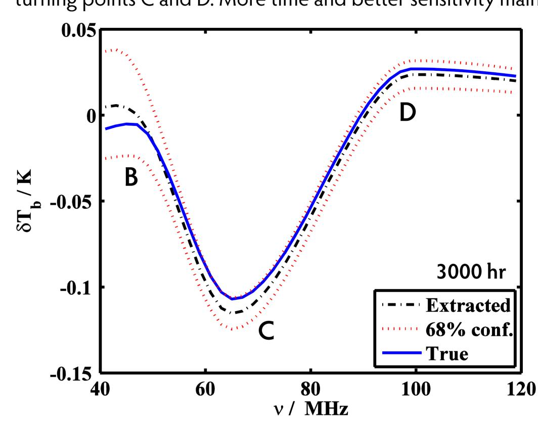
Inferred constraints on the 21-cm spectrum for the fiducial DARE mission. Uncertainties computed after marginalizing over all foreground and instrumental parameters. The frequencies of the turning points are very well constrained, and the errors on the temperatures are correlated: most of the uncertainty is in the overall normalization of the spectrum, not the shape.
