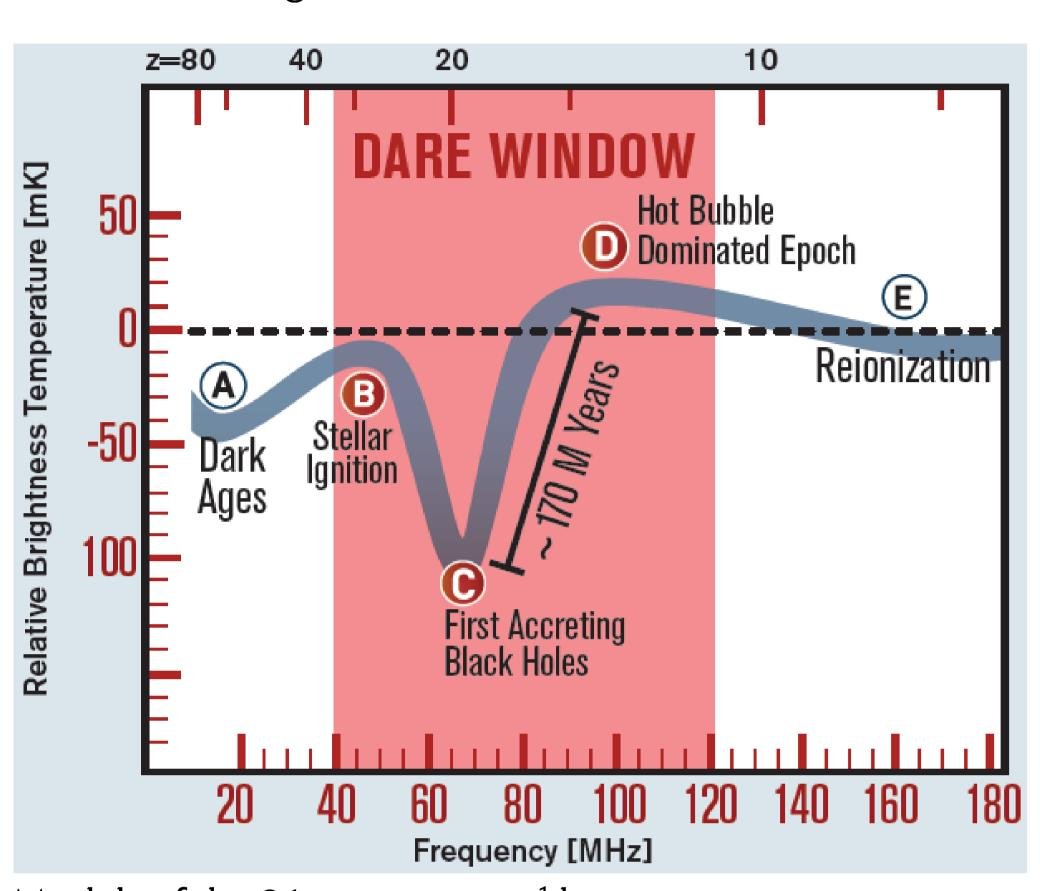
Models of the 21-cm spectrum<sup>1</sup> have turning points (A,B,C,D,E) whose positions encode the properties of the first sources of light in the Universe. The Dark Ages Radio Explorer (DARE) is an experiment to measure the position of turning points B,C and D from lunar orbit. A prototype for DARE is currently being deployed in Western Australia<sup>2</sup>, near the similar EDGES experiment.
